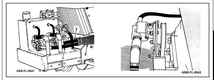
Attach the pressure hose (Item 1) ASM-FL-0042 from the auxiliary pump to the control valve (Item 1) ASM-FL-0042
